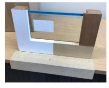
"Tricoya is a high performing wood fiberboard designed for environments of wet, high humidity or fully weather exposed applications. This would be applied on top of the existing wooden frames and cills."
