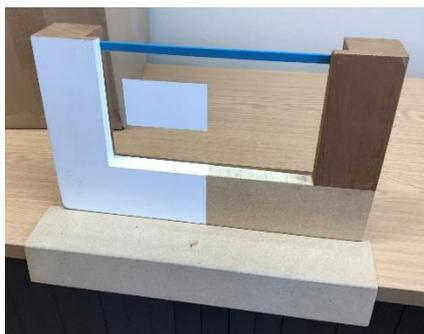
“Tricoya is a high performing wood fiberboard designed for environments of wet, high humidity or fully weather exposed applications. This would be applied on top of the existing wooden frames and cills.”
