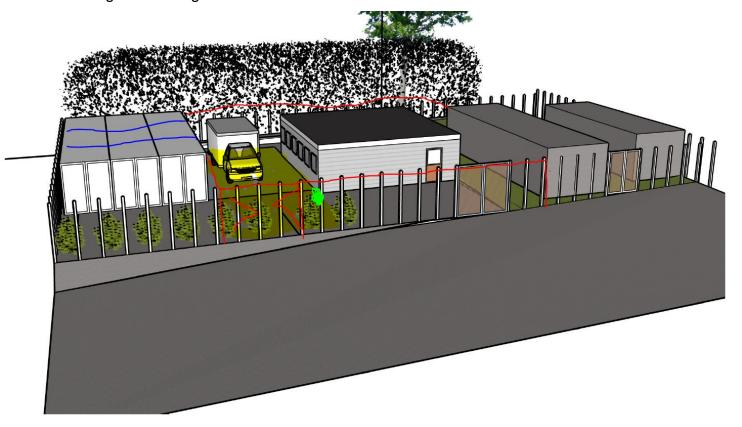
Red Line = Proposed revised reduced fencing and gate move Yellow shading = Type 2 hardstanding for van (some slope acceptable) Blue Line = rotate 90 degrees so easier to but on concrete pads
